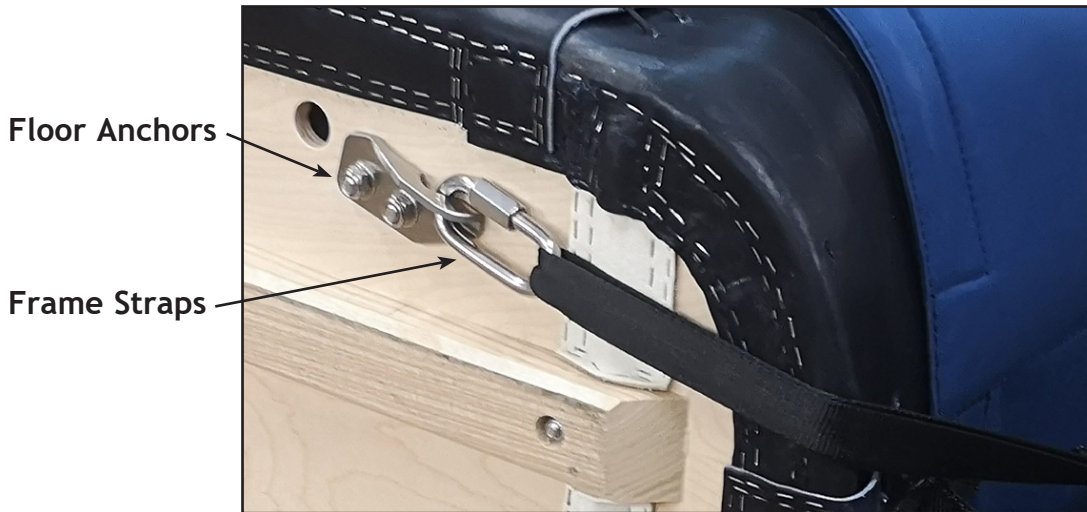
▲ Frame Strap attachment to Floor Anchor
