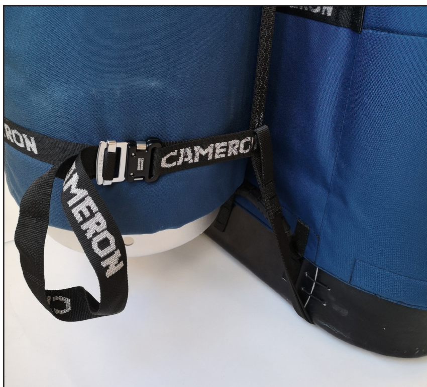
▲ Correct rigging of lower cylinder strap
