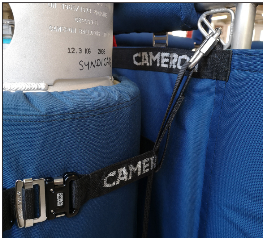
▲ Correct rigging of upper cylinder strap
