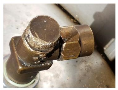
Fig 1. FLLG damaged by inappropriate use of tools.
