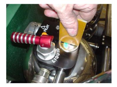
3. Use the Pressure gauge removal tool by pushing the small hooks down opposite sides of the gauge, then turn through 90° under the gauge bottom and pull the gauge out of the block. See picture below, if the burner is the opposite way up the gauge may fall out without the tools being necessary.
