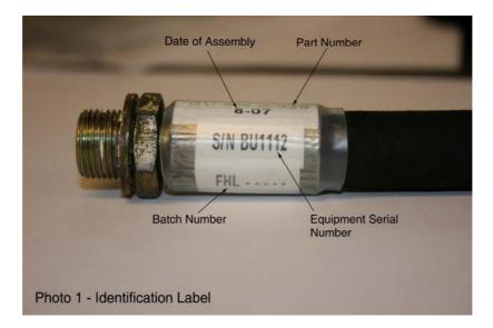
If the batch number begins with the three letters FHL then the hose must be inspected in accordance with the instructions under part 4. below.
